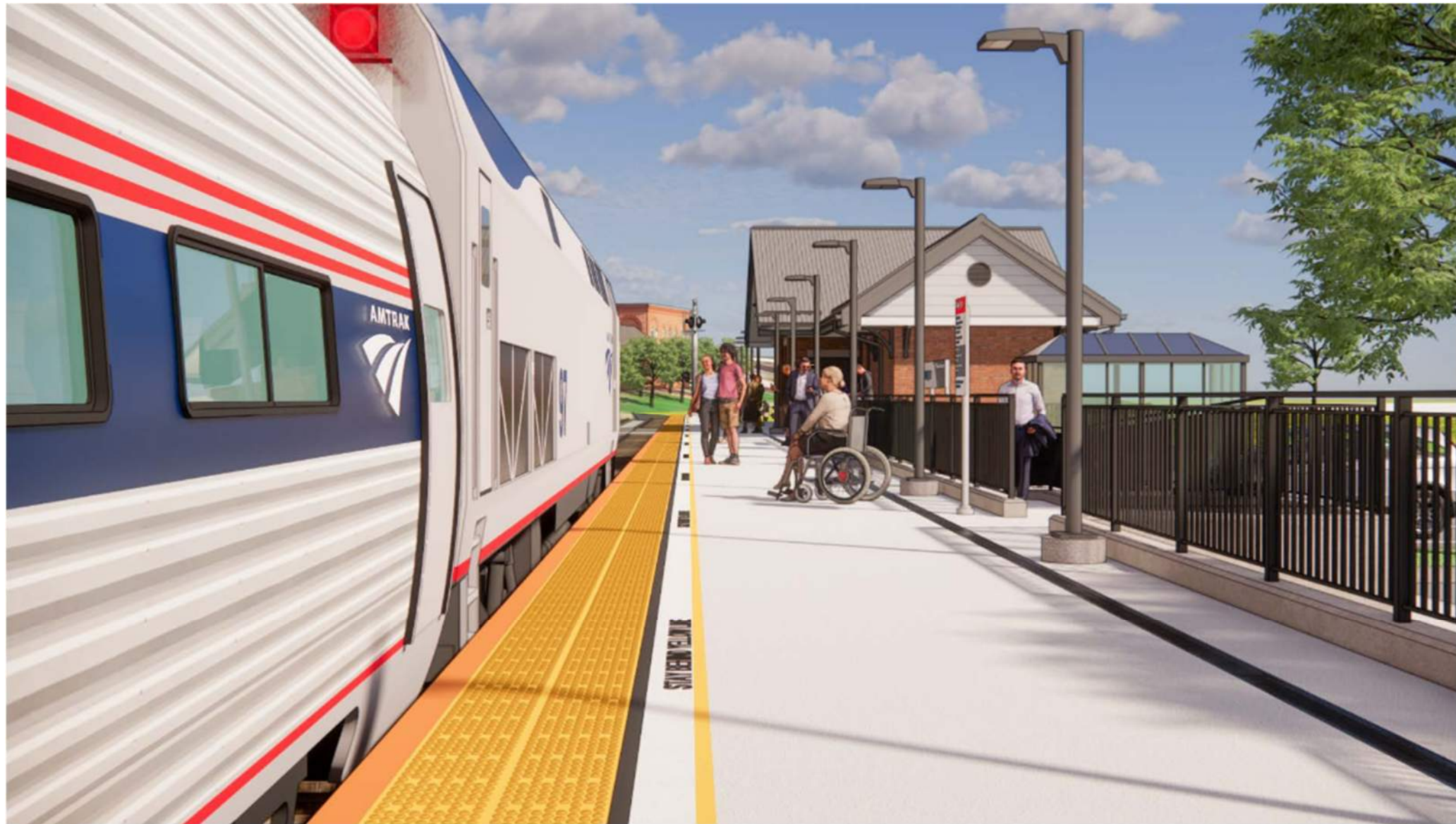
View from new 48 inch high platform looking north towards the new station building
