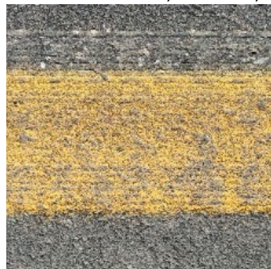
Recess Waterborne Paint, 8 months, 4-0+00
