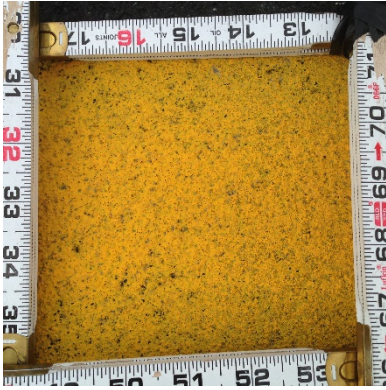
Surface MMA Wet Reflective, Installation, 9-0+00
