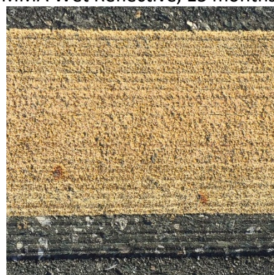
Recess MMA Wet Reflective, 15 months, 7-0+00
