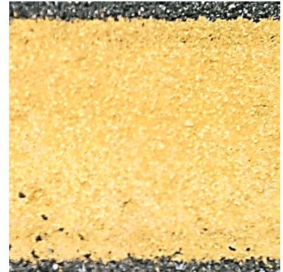
Surface Epoxy Wet Reflective, 36 months, 31-0+00
