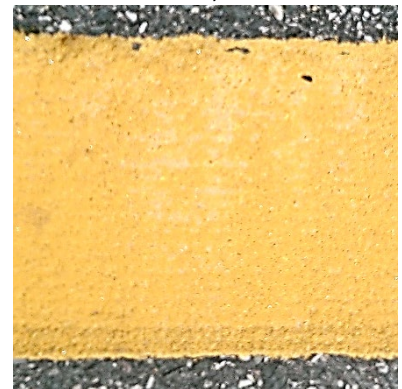
Recess Epoxy Utah, 36 months, 35-0+00
