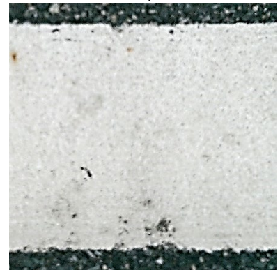
Recess Epoxy Wet Reflective, 36 months, 33-0+00
