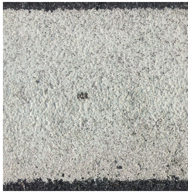
Surface Epoxy Wet Reflective, 15 months, 31-0+00
