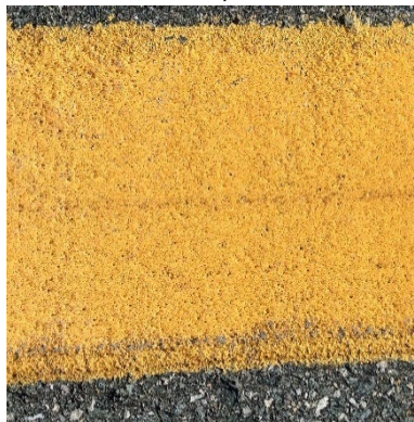
Recess Epoxy Utah, 15 months, 35-0+00
