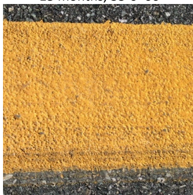
Recess Epoxy Wet Reflective, 15 months, 33-0+00
