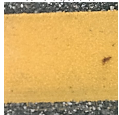
Recess Epoxy Wet Reflective, 36 months, 33-0+00
