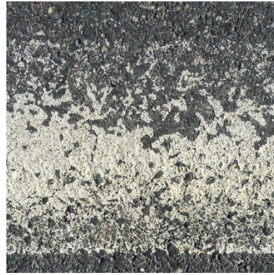
Surface MMA Wet Reflective, 15 months, 9-0+00
