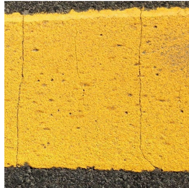
Surface Thermoplastic Utah, 8 months, 28-1+00
