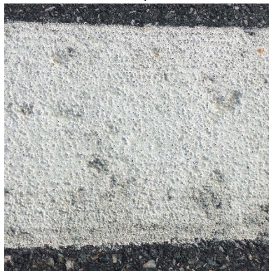
Recess Epoxy Wet Reflective, 15 months, 33-0+00
