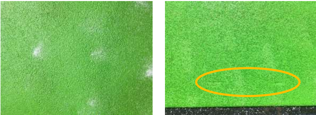
Figure 5: PreMark Skid Resistance (left) and Heat Indicator (right)
