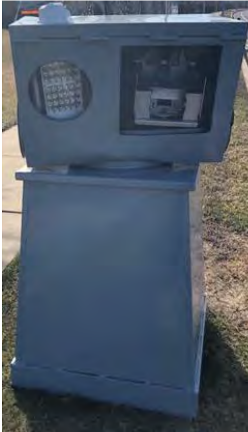
Figure 11 Camera System with Box Enclosure
