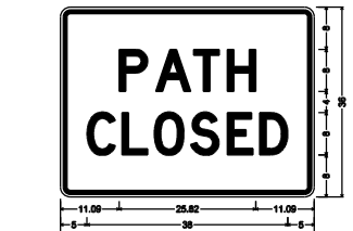
1.88" Radius, 0.75" Border, 0.50" Inset, Black on White; "PATH" D; "CLOSED" D specified length;
