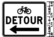
1.88" Radius, 0.75" Border, 0.50" Inset, Black on Orange; Symbol R0025; "DETOUR" D; Standard Arrow Custom 20.00" X 5.38" 180°;
