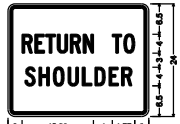
1.50" Radius, 0.65" Border, 0.38" Inset, Black on Orange; "RETURN TO" C specified length; "SHOULDER" C;
