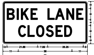
1.88" Radius, 0.75" Border, 0.50" Inset, Black on White; "BIKE LANE" D specified length; "CLOSED" D specified length;
