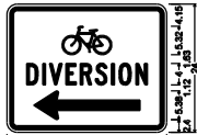
1.88" Radius, 0.75" Border, 0.50" Inset, Black on Orange; Symbol R0025; "DIVERSION" C; Standard Arrow Custom 20.00" X 5.38" 180°;
