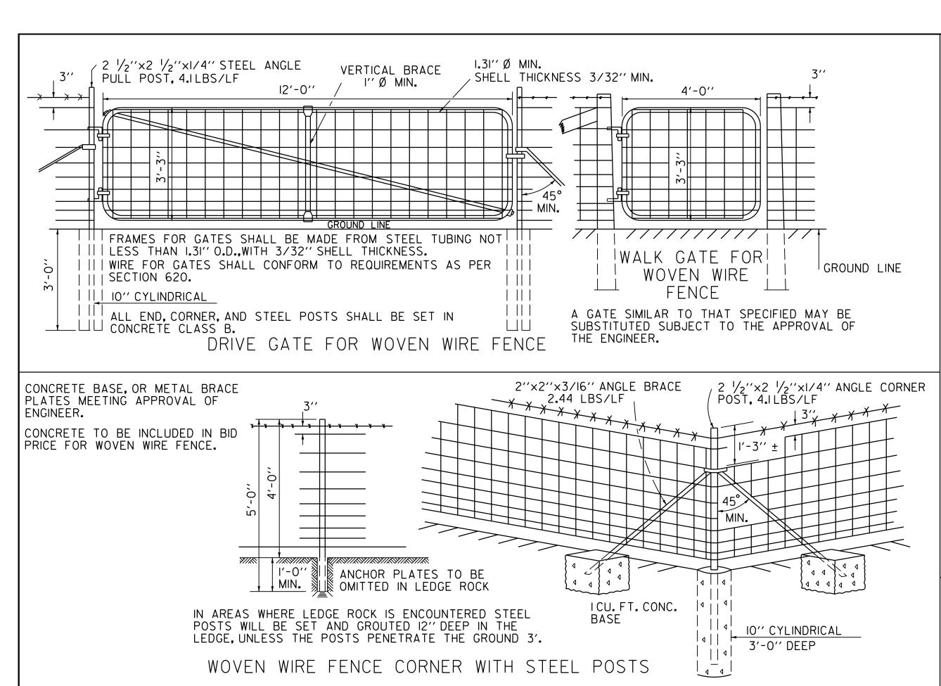
ALUMINUM COATED STEEL RECTANGULAR MESH OR GALVANIZED WOVEN RECTANGULAR MESH FENCE WITH NOT LESS THAN 9 HORIZONTAL BARS.
