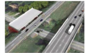
Step 3: Slide the new superstructure into place and reopen the bridge
