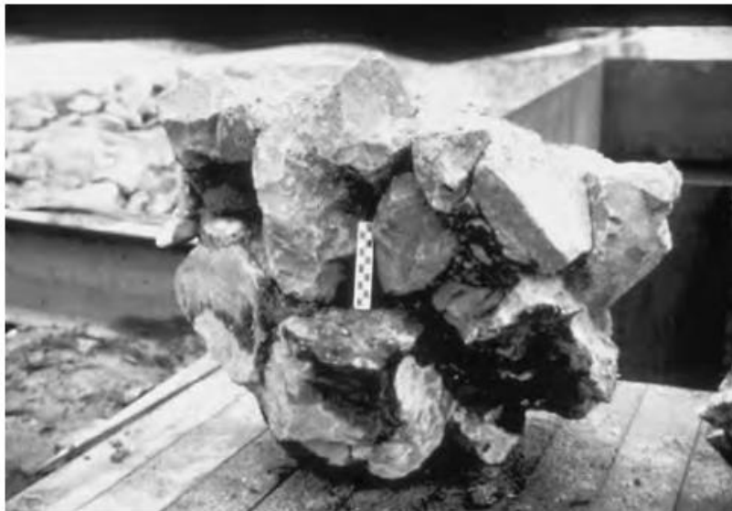
Figure 2.7: Partially grouted riprap aggregate (Lagasse et al, 2007)
