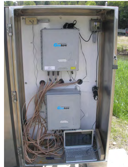
Figure 3-22: Data Acquisition System (Loggers) near Approach Slab
