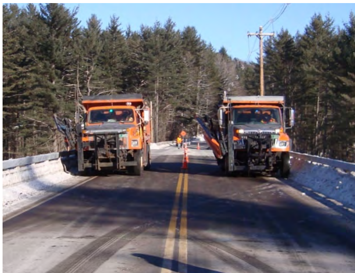
Figure 5-4: Middlesex Load Testing (Transverse Arrangement of Trucks)
