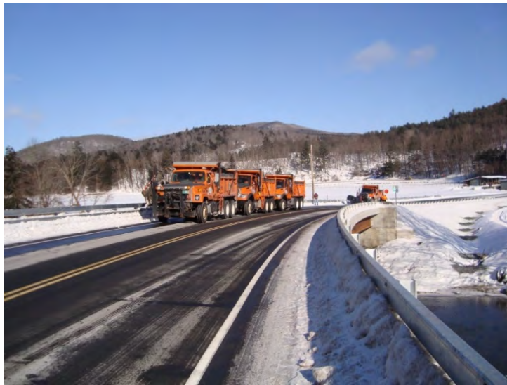
Figure 5-17: Stockbridge Bridge Load Testing
