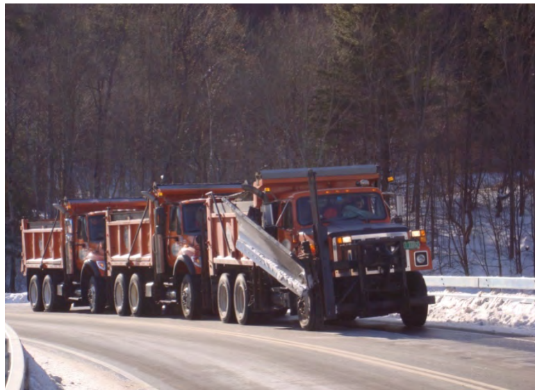
Figure 5-1: Load Testing of the Stockbridge Bridge
