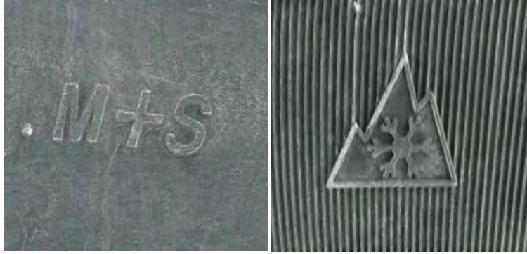
Figure 1. M+S (mud and snow) symbol on all season tires (left) and snow and mountain symbol found on winter tires.
