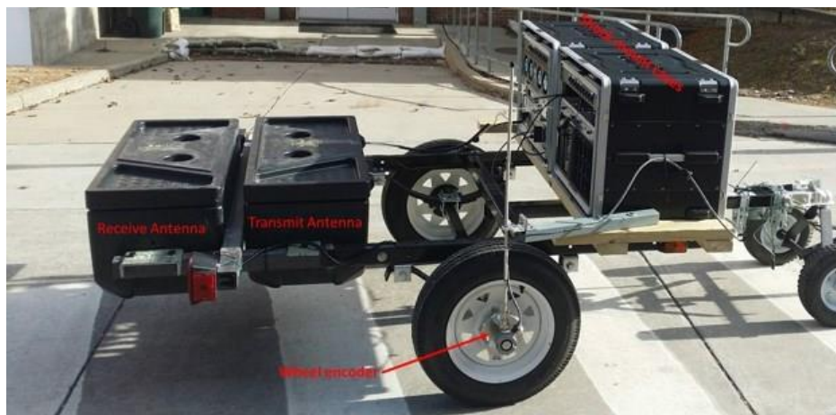
Fig. 10. UVM GPR System mounted on a trailer
