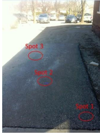
Fig. 20 Asphalt Pavement Dielectric Constant Monitoring Test Spots
