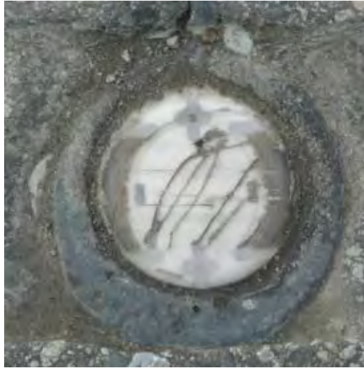
FIGURE 8 Damage to LED.
