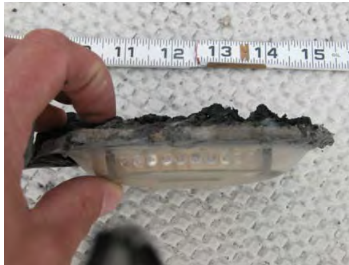
FIGURE 4 LED after removal.
