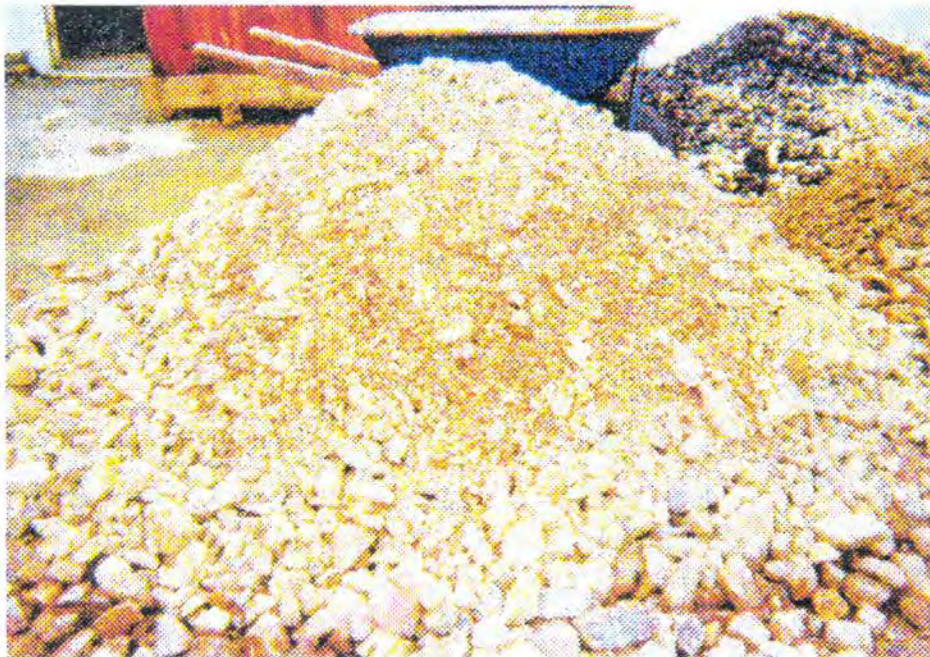
Fine dense graded crushed stone provided by Whitcomb Construction Co., Winooski, VT
