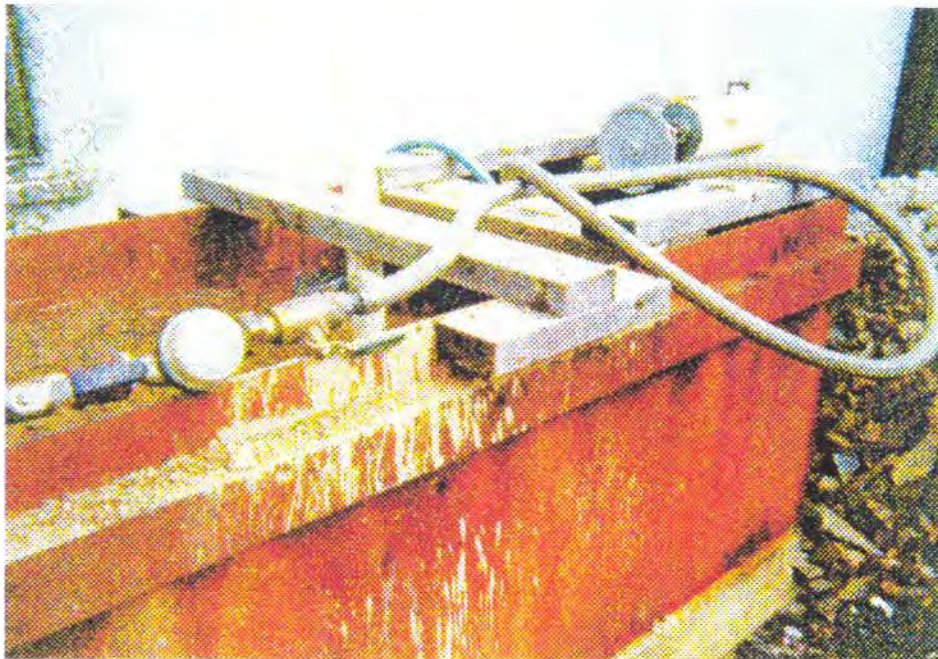
Horizontal permeability testing apparatus showing reservoir controls and flow metering device
