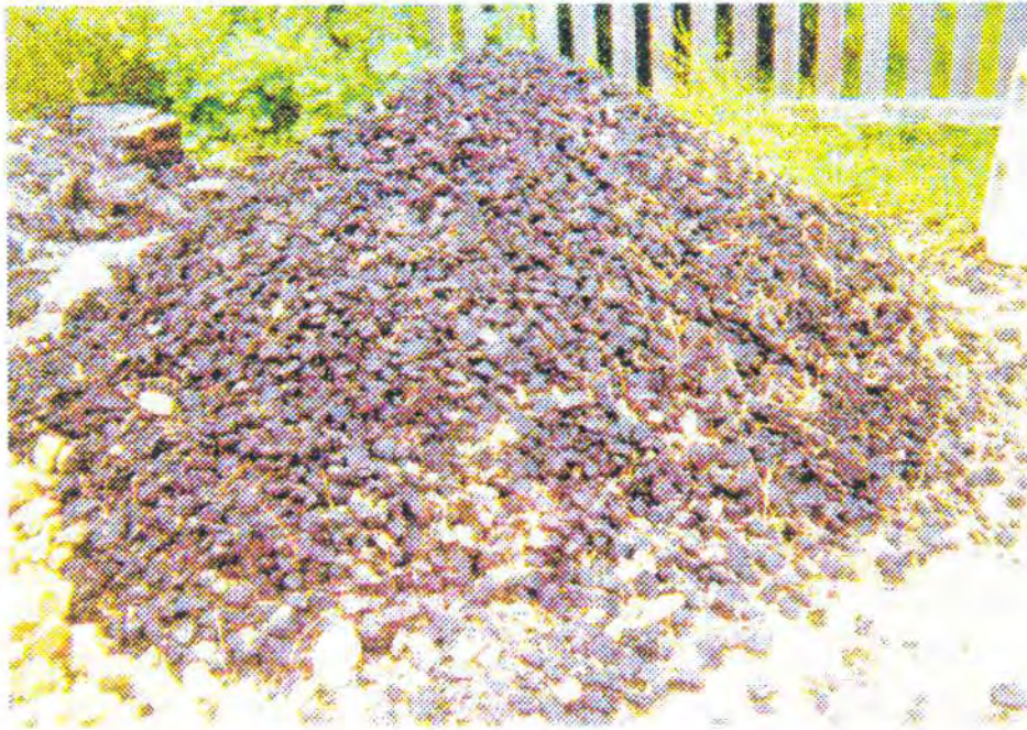
Asphalt-treated permeable base course provided by Pike Industries, Williston, VT
