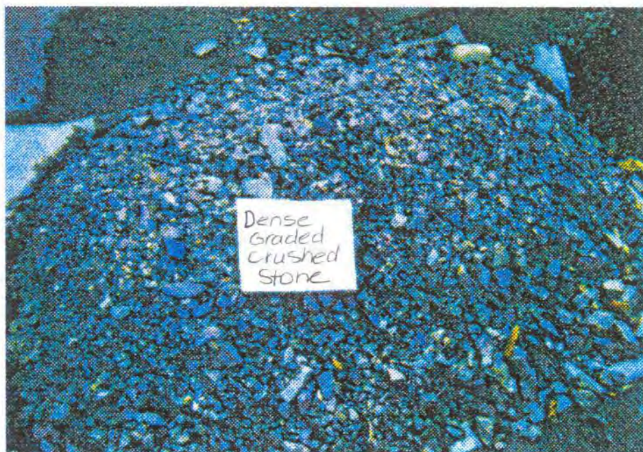
Dense graded crushed stone provided by Whitcomb Construction Co., Winooski, VT.
