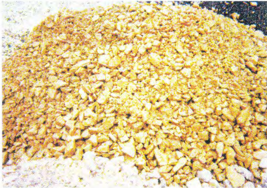
Coarse dense graded crushed stone provided by Whitcomb Construction Co., Winooski, VT
