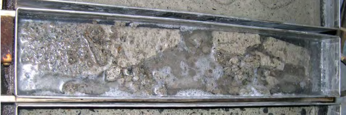
Figure 7a: Sample prior to removal from freeze-thaw apparatus.
