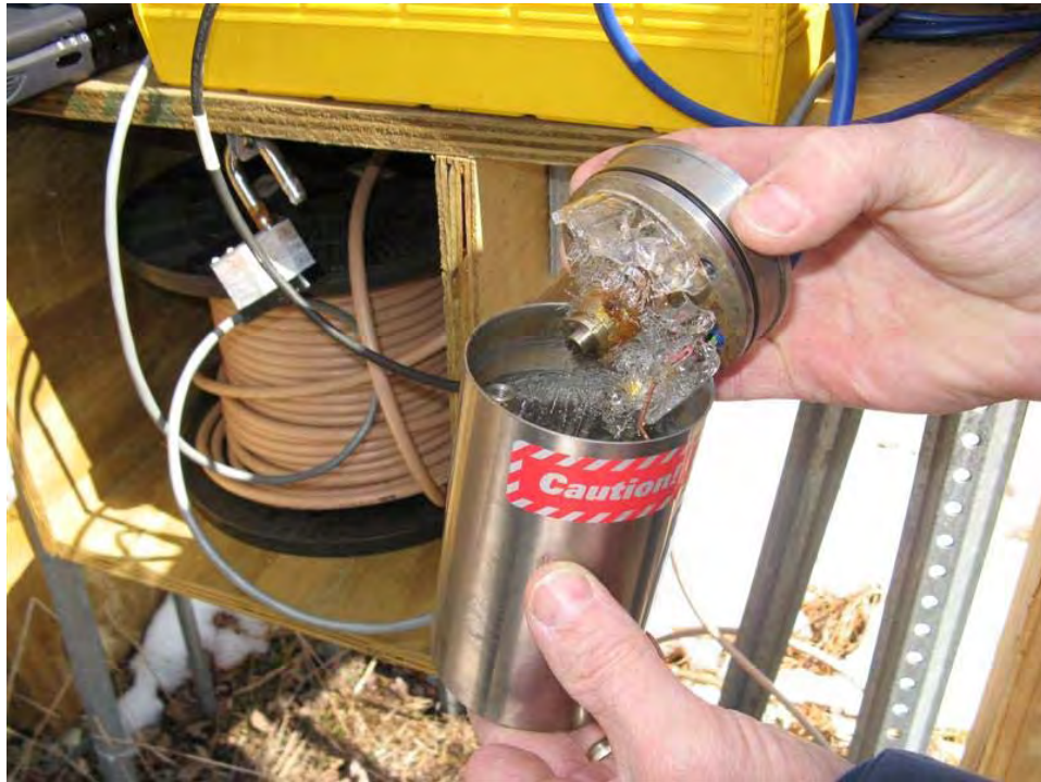
Figure 3.6 Ice damage inside the sealed barometer.
