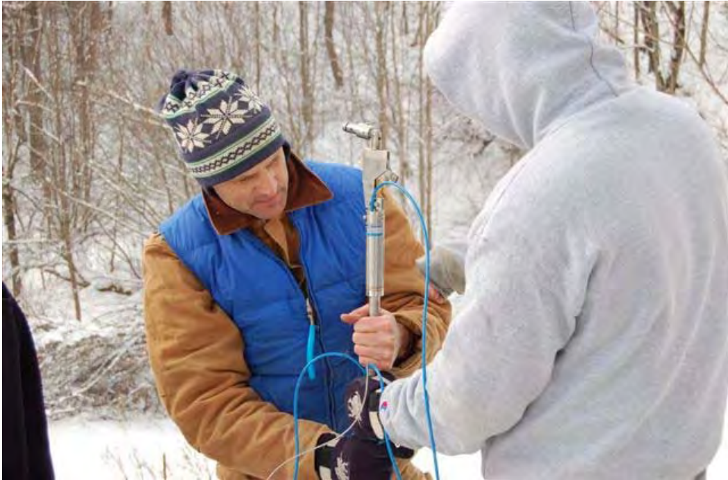
Figure 3.3 Installing an IPI.
