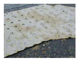
The remaining portion of this product showed extreme fading of the color and damage to domes. This product failed.
