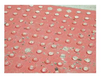
Based on the continued damage observed with this product each winter, it is considered to have failed. A three year life span for these materials is not acceptable.
