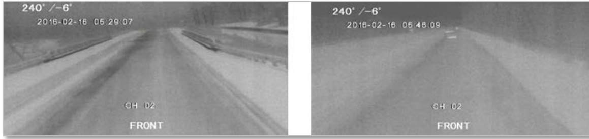
Figure 18 Image Quality Degradation Caused by Buildup on the Camera Lens
