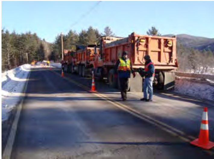
Figure 5-2: Middlesex Load Testing (Longitudinal Arrangement of Trucks)
