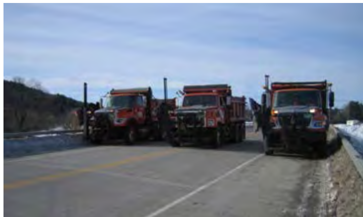
Figure 5-12: East Montpelier Load Testing (Transverse Arrangement of Trucks)
