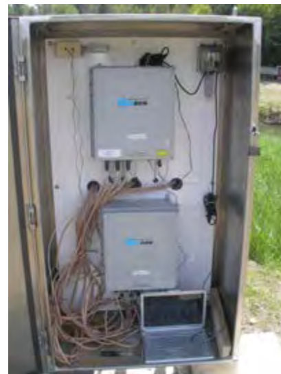
Figure 3-22: Data Acquisition System (Loggers) near Approach Slab
