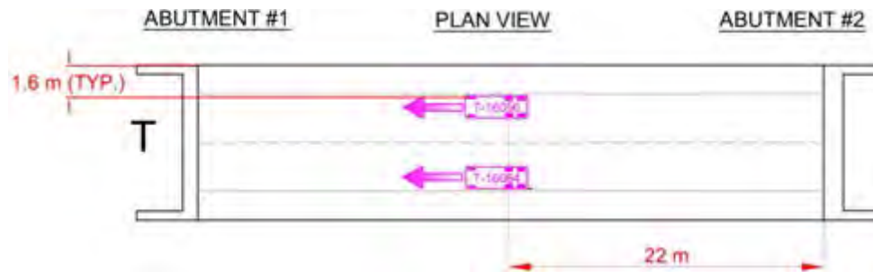
Figure 5-8: Middlesex Load Testing Truck Locations (Transverse Arrangement)
