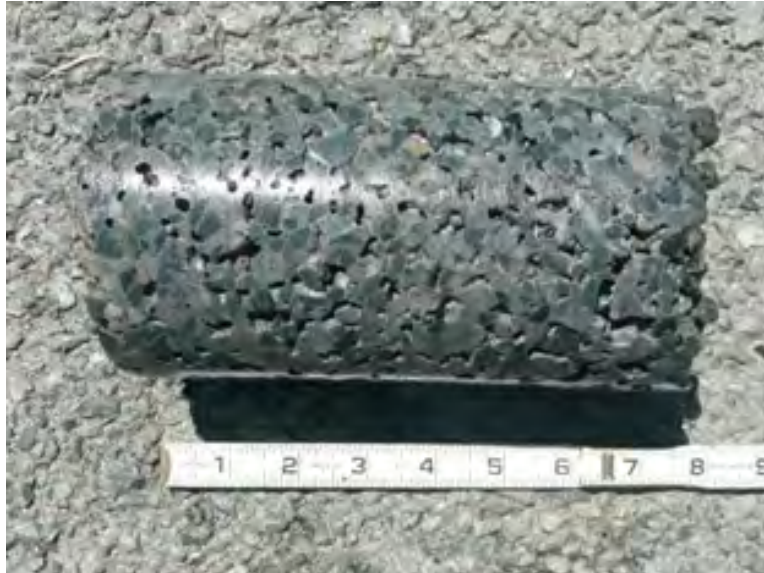
Figure 10. Core 6, taken from a visually and audibly sound but clogged location at the exit.
