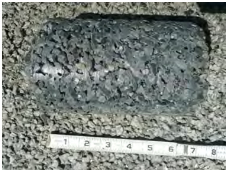
Figure 7. Core 3, taken from a visually and audibly sound location, two feet from Core 2.
