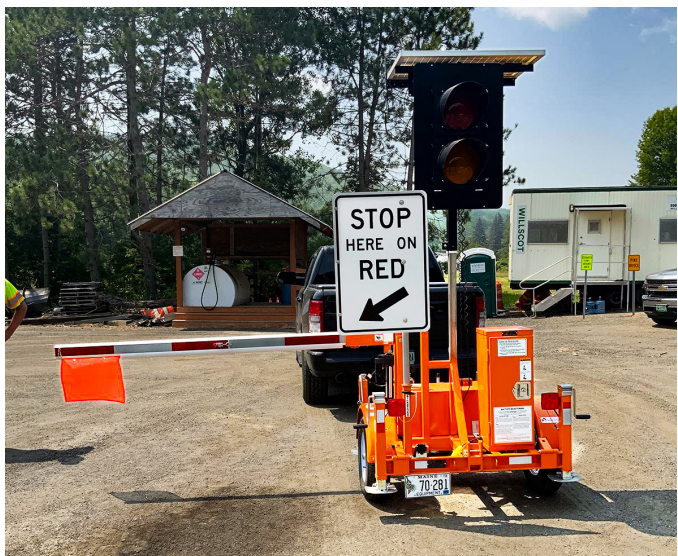
Travelers encountered a new safety technology on the roadway this construction season: Automated Flagger Assistance Devices, or AFADs, are mechanically controlled flagging devices that allow human flaggers to stay out of the roadway while managing the flow of traffic, improving safety for workers and motorists alike.
