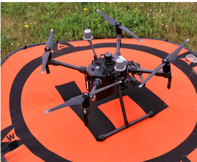
UNMANNED AERIAL SYSTEMS. AOT’s UAS program continues to grow and improve. The newest drone connects to as many as 27 different satellites at one time for extremely accurate mapping imagery, which can be used to create 3D models of terrain, obstructions, and structures.
