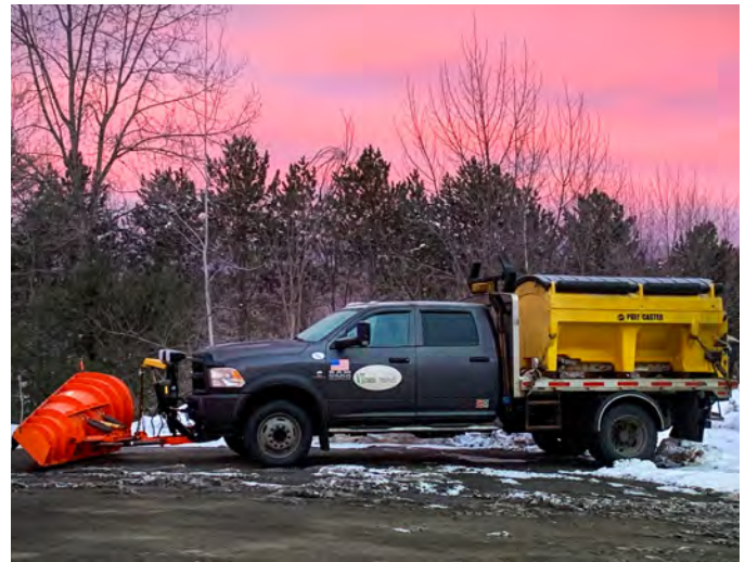
RANDOLPH. While the big orange trucks might be the most iconic VTrans vehicle, other smaller trucks are also equipped with plows and road treatment materials to assist with winter maintenance.
