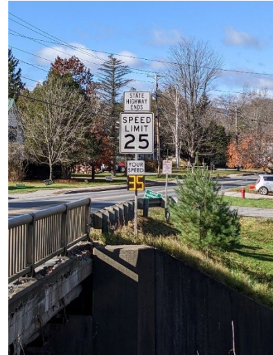
Figure 4. Application of a dynamic radar speed feedback sign in Vermont.
