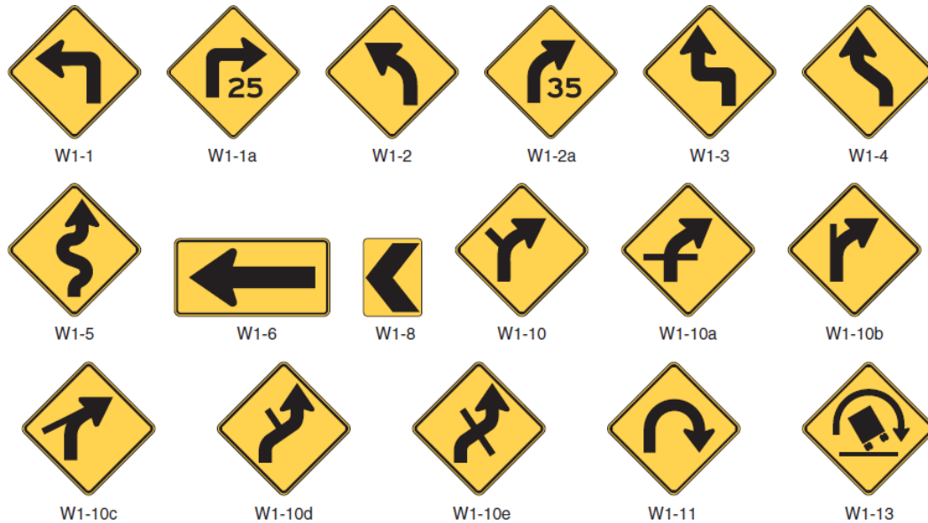
Figure 3. Curve warning signs per the MUTCD. [Source: MUTCD Figure 2C-1]
