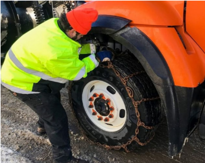
Weighing in at almost 60,000 lbs per vehicle, VTrans plow trucks need every safety advantage they can get. Chaining up plow tires is common practice to ensure drivers have the best traction possible when battling the winter elements.
