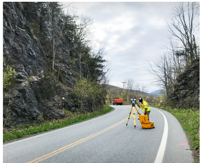
POWNA. VTrans Survey field crew members use 3D Terrestrial LiDAR scanners to monitor movement in at-risk rock ledges along Vermont roadways. These static laser scanners record light pulses at a rate of one million points per second to create a 3D model of whatever feature or structure is being scanned. Those models are referenced into the Vermont State Plane coordinate system and are used in the design and planning process for transportation projects.
