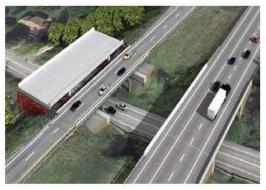
Step 3: Slide the new superstructure into place and reopen the bridge
