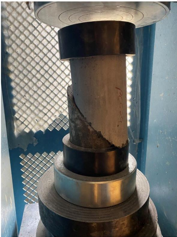
**Figure 3-6: Bond Shear Strength Specimen**
