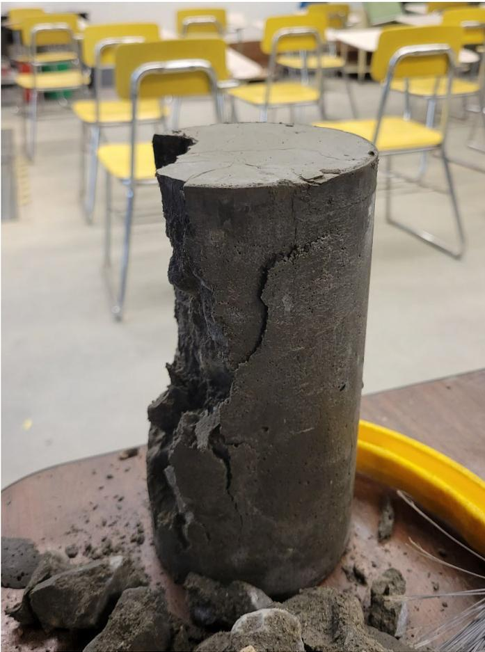
**Figure 3-5: Compressive Strength Test Specimen After Failure**
