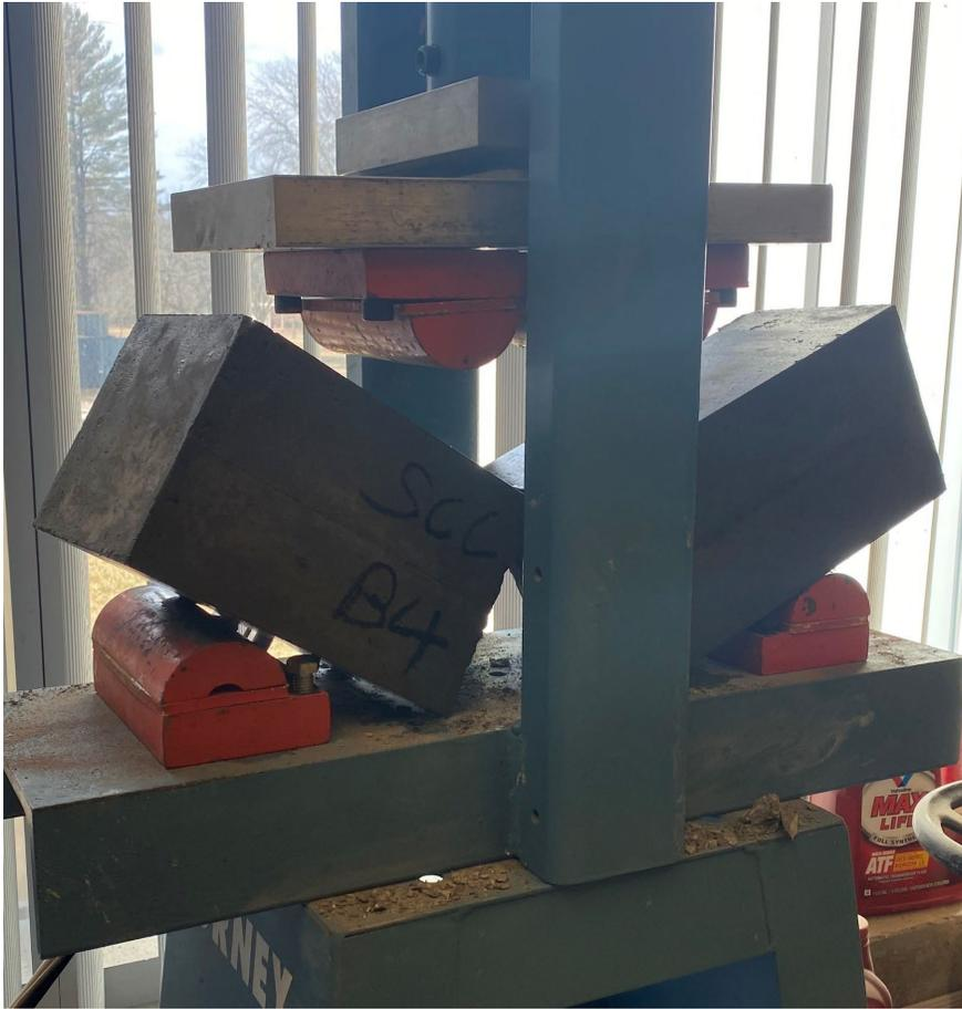
**Figure 3-4: Flexural Strength Test**
