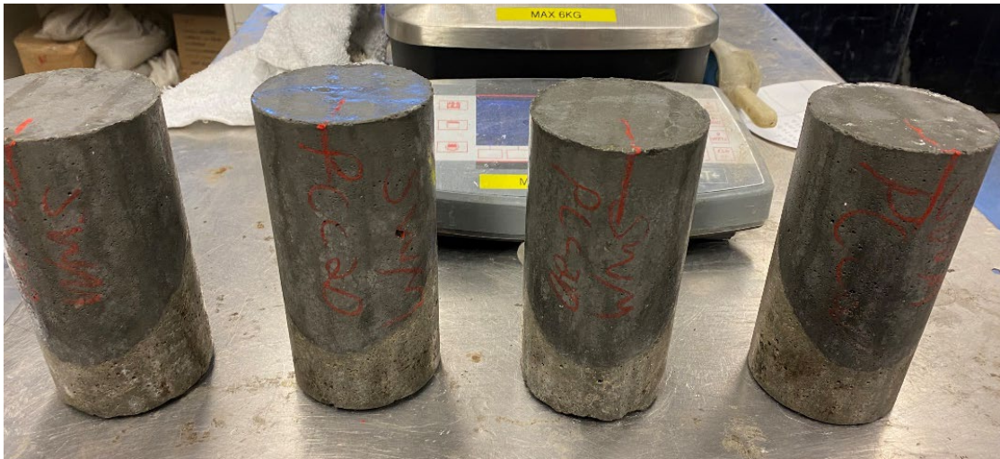
Figure 4-13: Mix Iteration PCC-2d Bond Shear Strength Specimens After Conditioning
