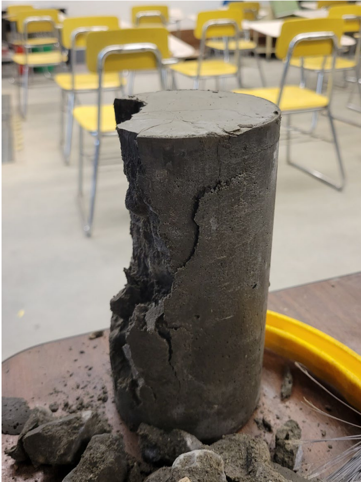
Figure 3-5: Compressive Strength Test Specimen After Failure
