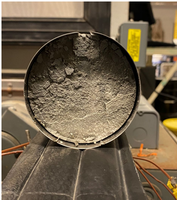
Figure 3-8: Stainless Steel Mold for Freeze Thaw Conditioning Chamber with Cylindrical Specimen Inserted
