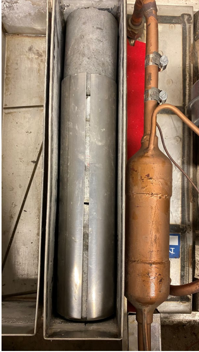
Figure 3-9: Stainless Steel Mold for Freeze Thaw Conditioning Chamber Placed Inside Freeze Thaw Chamber
