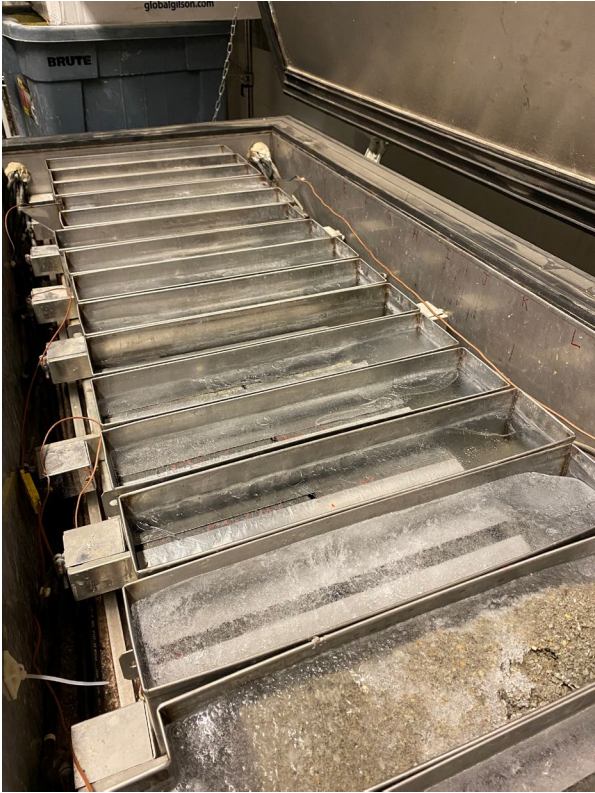
Figure 3-10: Freeze Thaw Conditioning Chamber with Specimens Undergoing Conditioning
