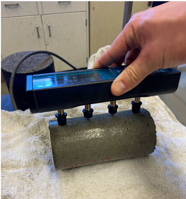
Figure 3-11: Surface resistivity test
