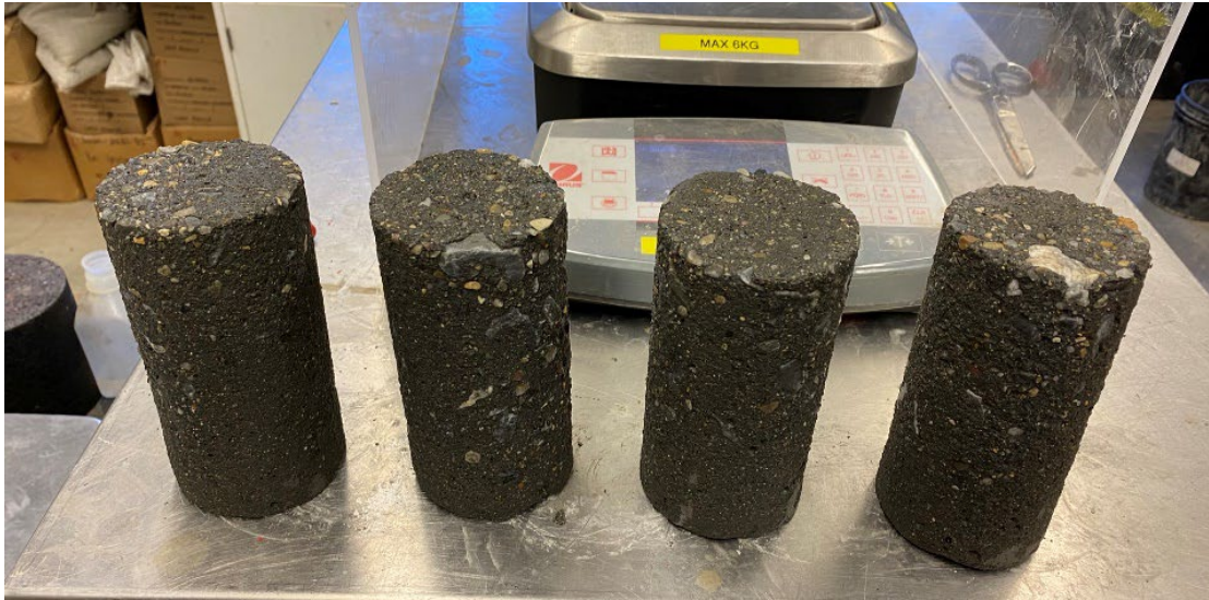
Figure 4-11: Mix Iteration PCC-2d Compressive Strength Specimens After Conditioning
