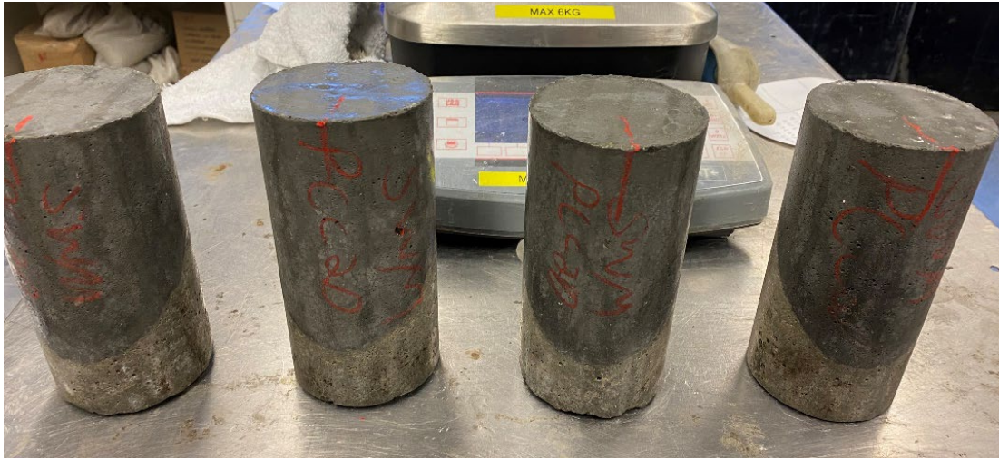
Figure 4-12: Mix Iteration PCC-2d Bond Shear Strength Specimens Before Conditioning
