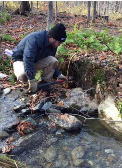
Figure 3: Soil sampling. Left panel displays technician collecting a soil sample with AMS soil coring device. Right panel displays sample collection approach, with samples collected along the gully wall, at 30 cm depths.
